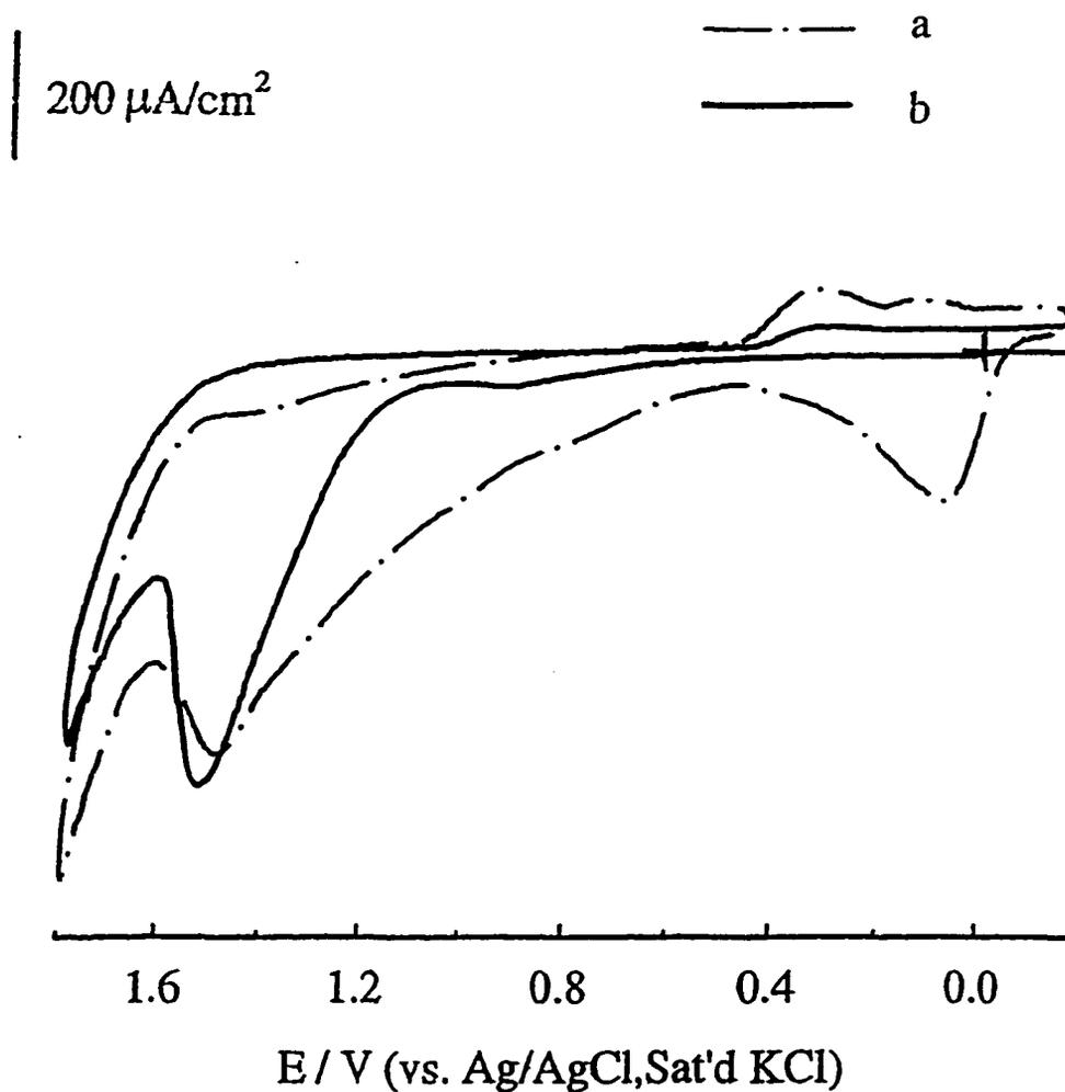
**Figure 10.** Cyclic voltammograms obtained at freshly polished GCEs in aqueous 0.5 M  $LiClO_4$  solutions containing (a) 0.2 mM dopamine, (b) solution a plus 0.4 mM  $CoCl_2$ . The pH values of solutions were adjusted to 9.6 before potential scannings. The applied voltage was cycled once between 0.00 V and +1.80 V at 10 mV/s in each case.
