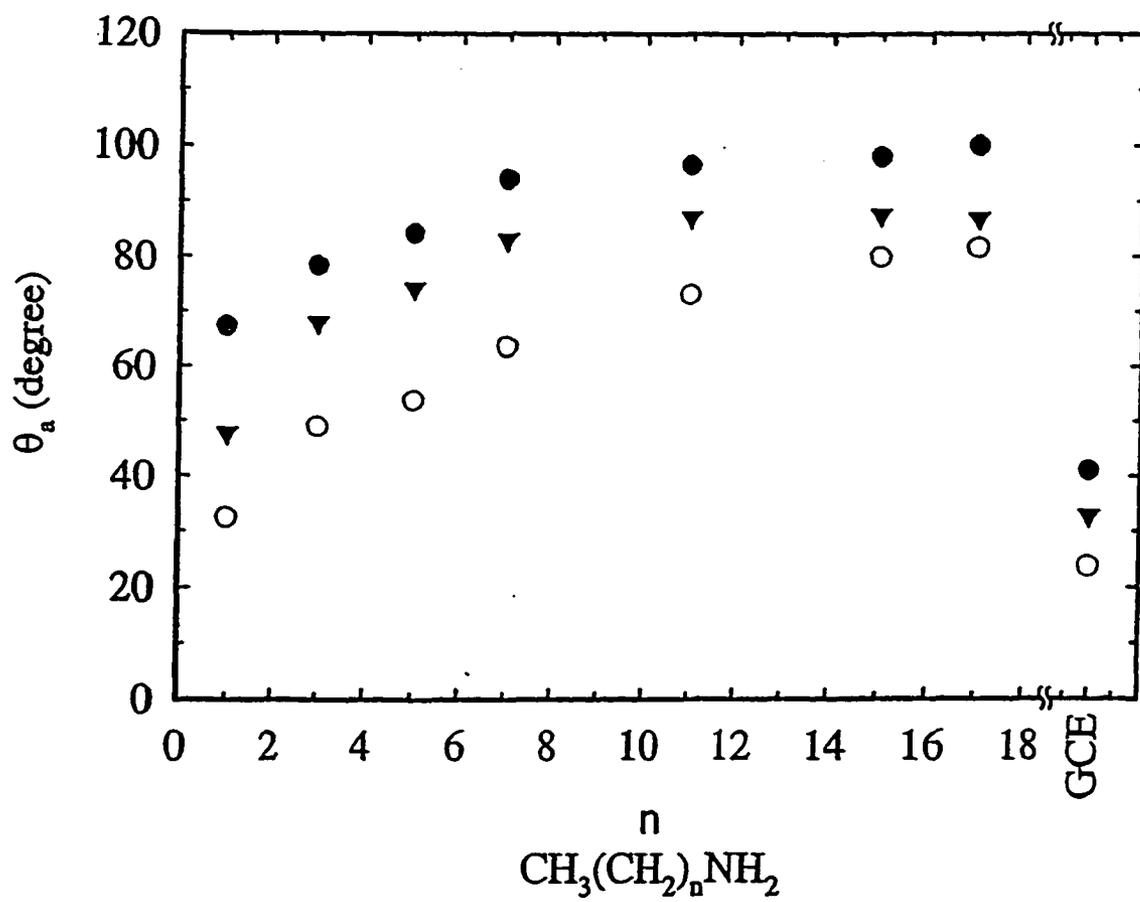
Figure 5. Advancing contact angles of formamide ( $\circ$ ), glycerol ( $\blacktriangledown$ ) and water ( $\bullet$ ) for alkylamine ( $\text{CH}_3(\text{CH}_2)_n\text{NH}_2$ ) modified GCE surface. GCE = freshly polished GCE surface.
