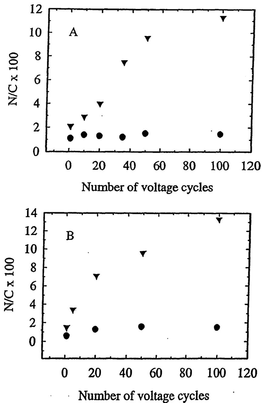
**Figure 2.** Variation of N/C values with the number of voltage cycles for the immobilization of amines on GCEs in 0.1 M  $\text{NBu}_4\text{BF}_4$  ethanolic solutions (●) or methylene chloride solutions (▼) containing 2mM (A) *N*-ethylbutylamine, and (B) triethylamine. The applied voltage scanned between 0.00 V and +1.80 V at 10 mV/s.
