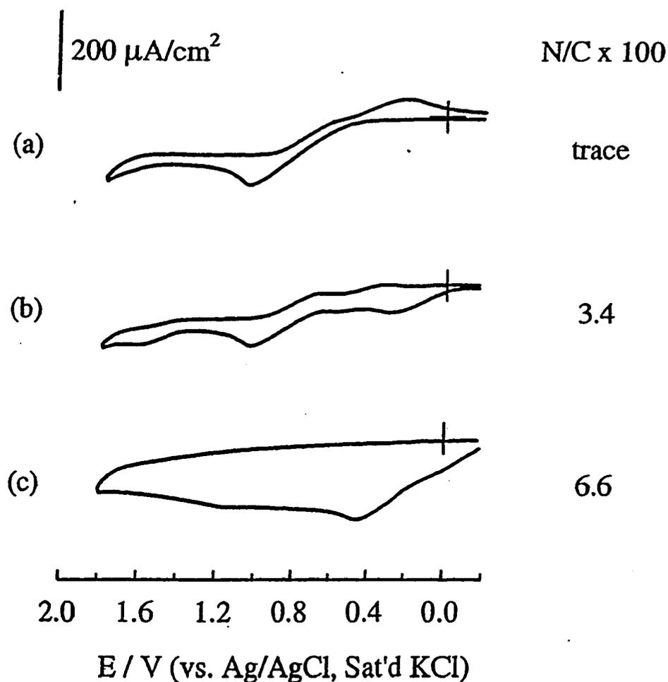
**Figure 8.** Cyclic voltammograms obtained at freshly polished GCEs immersed in ethanolic 0.1 M LiClO<sub>4</sub> solutions (ethanol:water, 100:1 (v/v) containing (a) 2 mM dopamine hydrochloride (DA) only, (b) solution a plus 2.0 mM LiOH, and (c) solution a plus 6.0 mM LiOH. The applied voltage was cycled once between -0.10 V and +1.80 V at 10 mV/s in each case.
