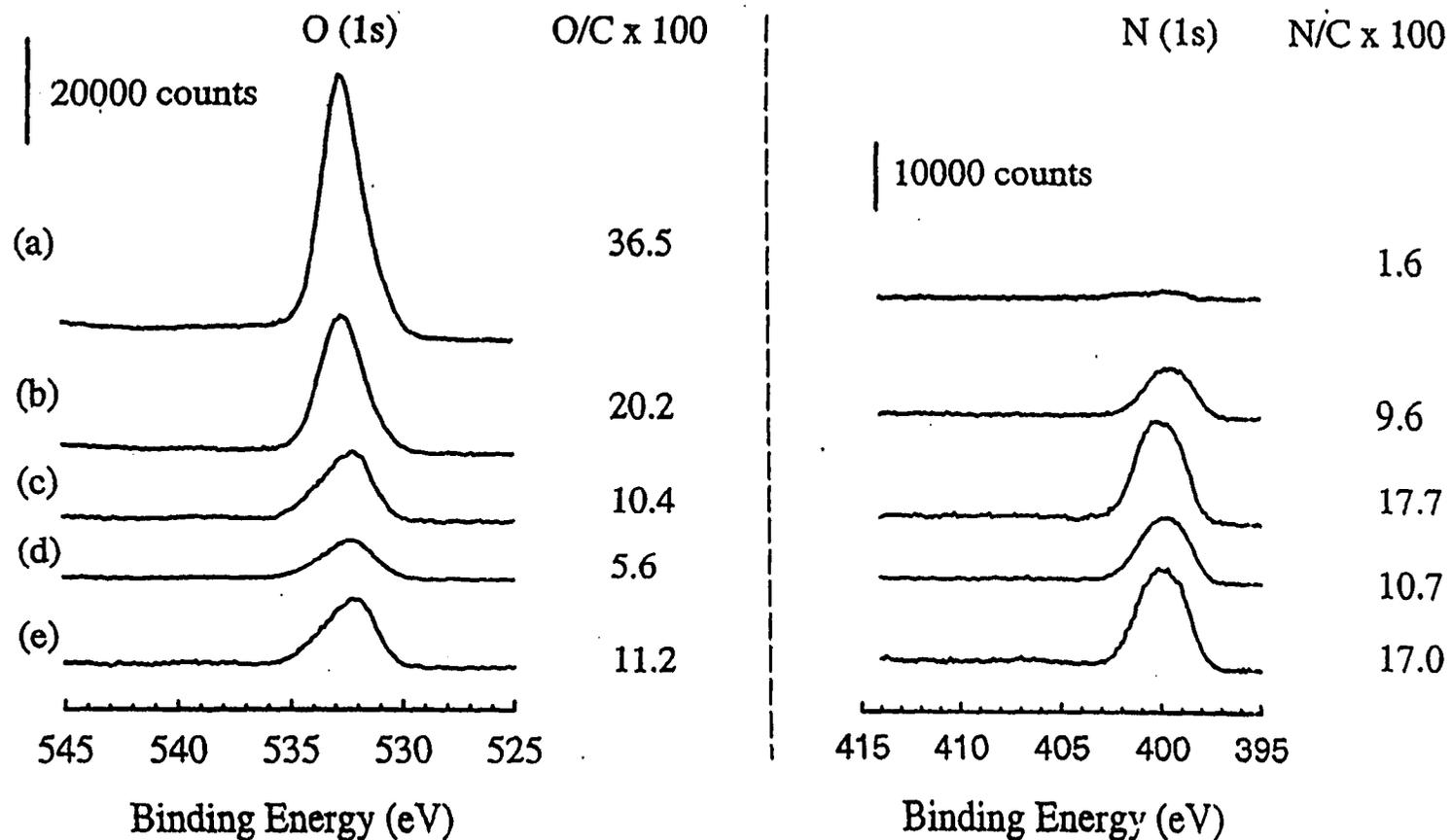
**Figure 4.** X-ray photoelectron spectra in the O(1s) and N(1s) region for (a) electrochemical pretreated GCE and (b) freshly polished GCE immersed in an ethanolic solution, (c) freshly polished GCE and (d) vacuum heat treated GCE in an acetonitrile solution, (e) vacuum heat treated GCE in an mixed solution of acetonitrile and water (ACN:H<sub>2</sub>O ; 100:1 (v/v) ) containing 2 mM phenethylamine. In each case, the applied voltage was cycled 5 times between 0.00 V and +1.80 V at 10 mV/s.
