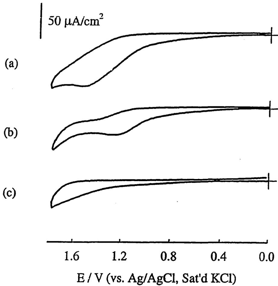
**Figure 6.** Cyclic voltammograms obtained at freshly polished GCEs in ethanolic 0.1 M  $\text{LiClO}_4$  solutions (ethanol:water; 100:1 (v/v) ) containing (a) 2 mM phenethylamine (PA) only, (b) solution a plus 1.0 mM  $\text{HClO}_4$ , and (c) solution a plus 3.0 mM  $\text{HClO}_4$ . The scan rate was 10 mV/s.
