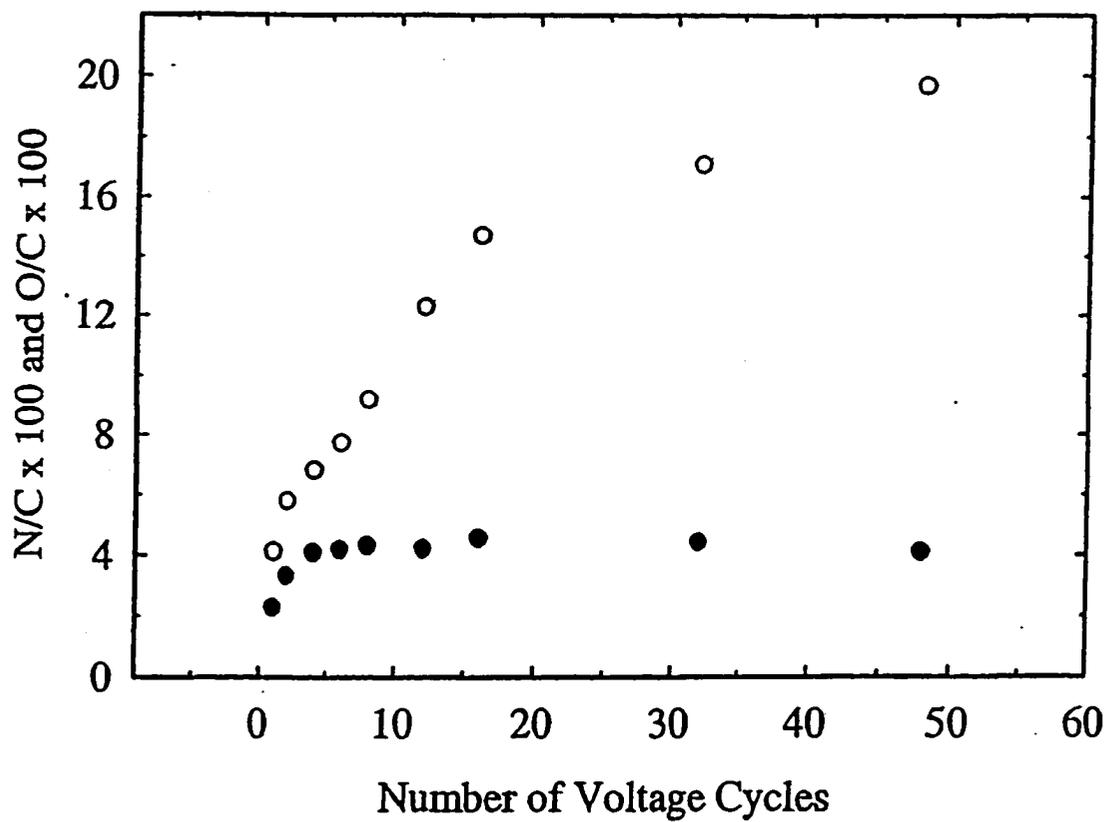
**Figure 6.** Variation of N/C (●) and O/C (○) values with the number of voltage cycles for immobilization of GC electrodes in 0.1 M LiClO<sub>4</sub> ethanolic solutions containing 4 mM octadecylamine with the applied voltage scanned between 0.00V and +1.80 V for different cycles. The scan rate was 10 mV/s.
