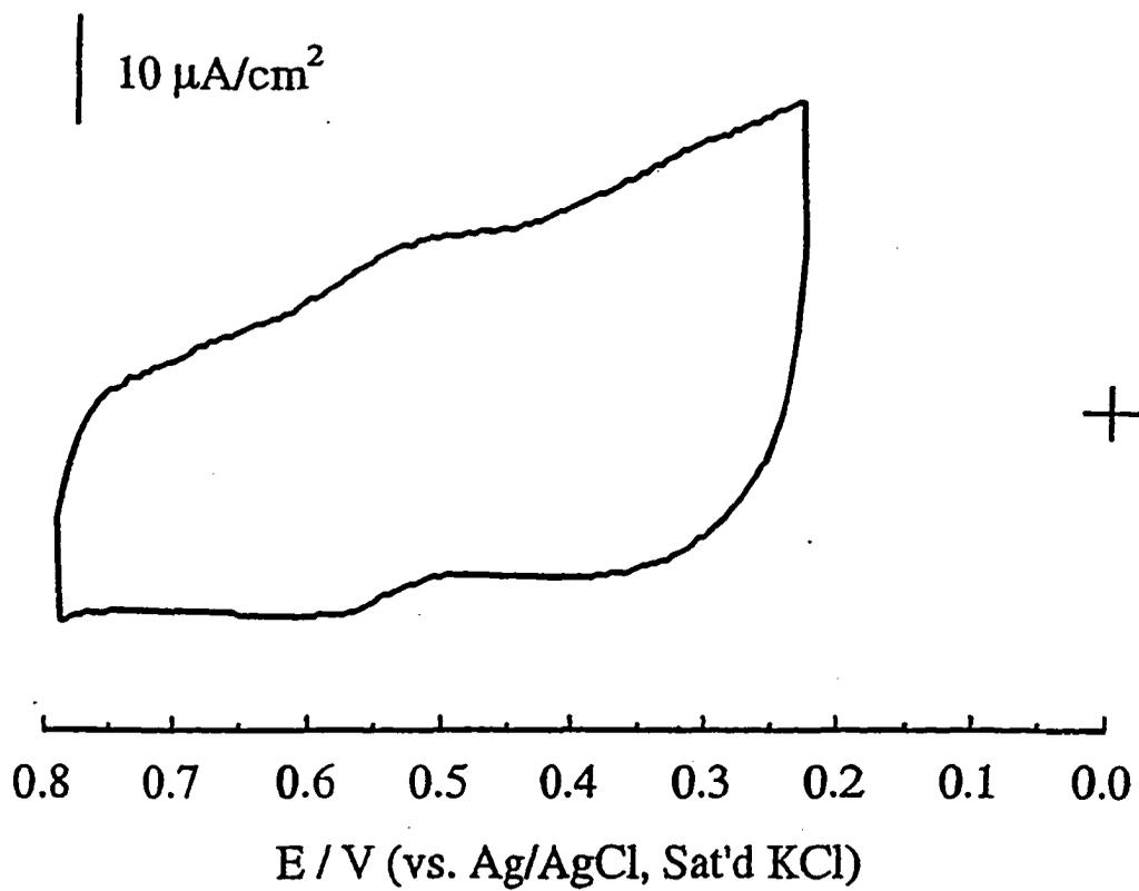
**Figure 9.** Cyclic voltammogram obtained in aqueous 0.1 M HClO<sub>4</sub> at a DA-modified GCE from Figure 8c. The scan rate was 100 mV/s.
