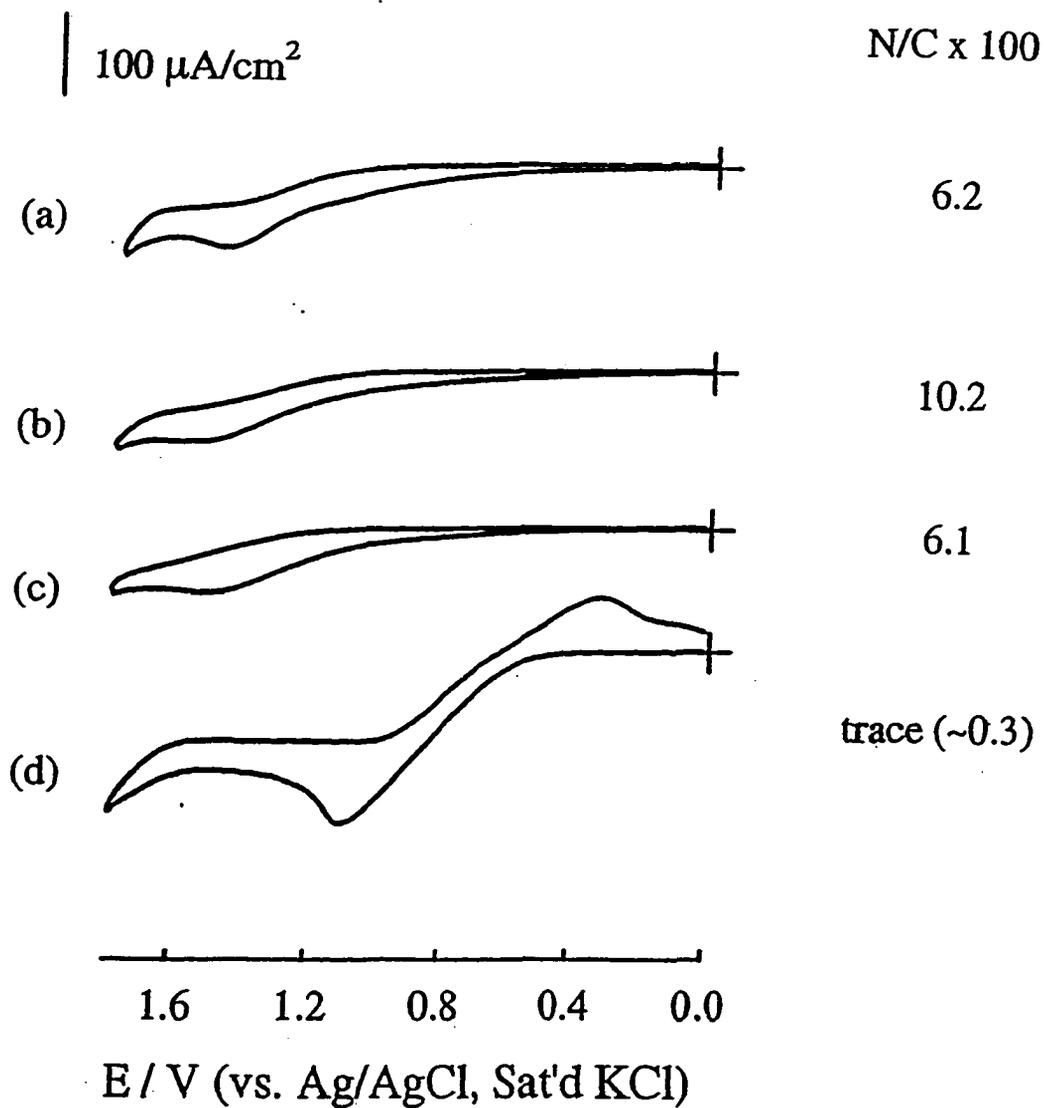
**Figure 5.** Cyclic voltammograms and N/C values obtained at freshly polished GCEs in ethanolic 0.1 M  $\text{LiClO}_4$  solutions containing 2 mM of (a) butylamine, (b) *N*-acetylenediamine, (c) phenethylamine, and (d) dopamine hydrochloride. The scan rate was 10 mV/s in each case.
