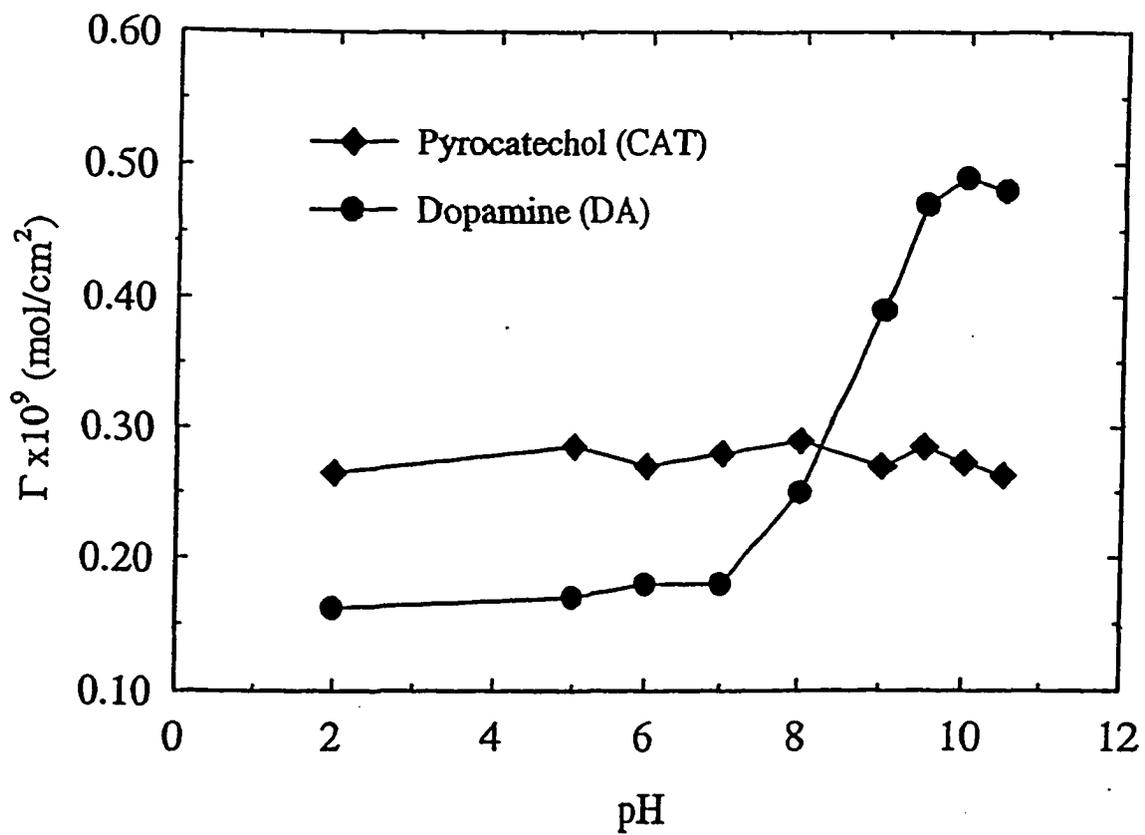
Figure 4. Adsorption data for CAT and DA on GCEs, expressed as  $\Gamma$  ( $\text{mol cm}^{-2}$ ), as a function of solution pH. The solid lines serve only to connect the experimental data.
