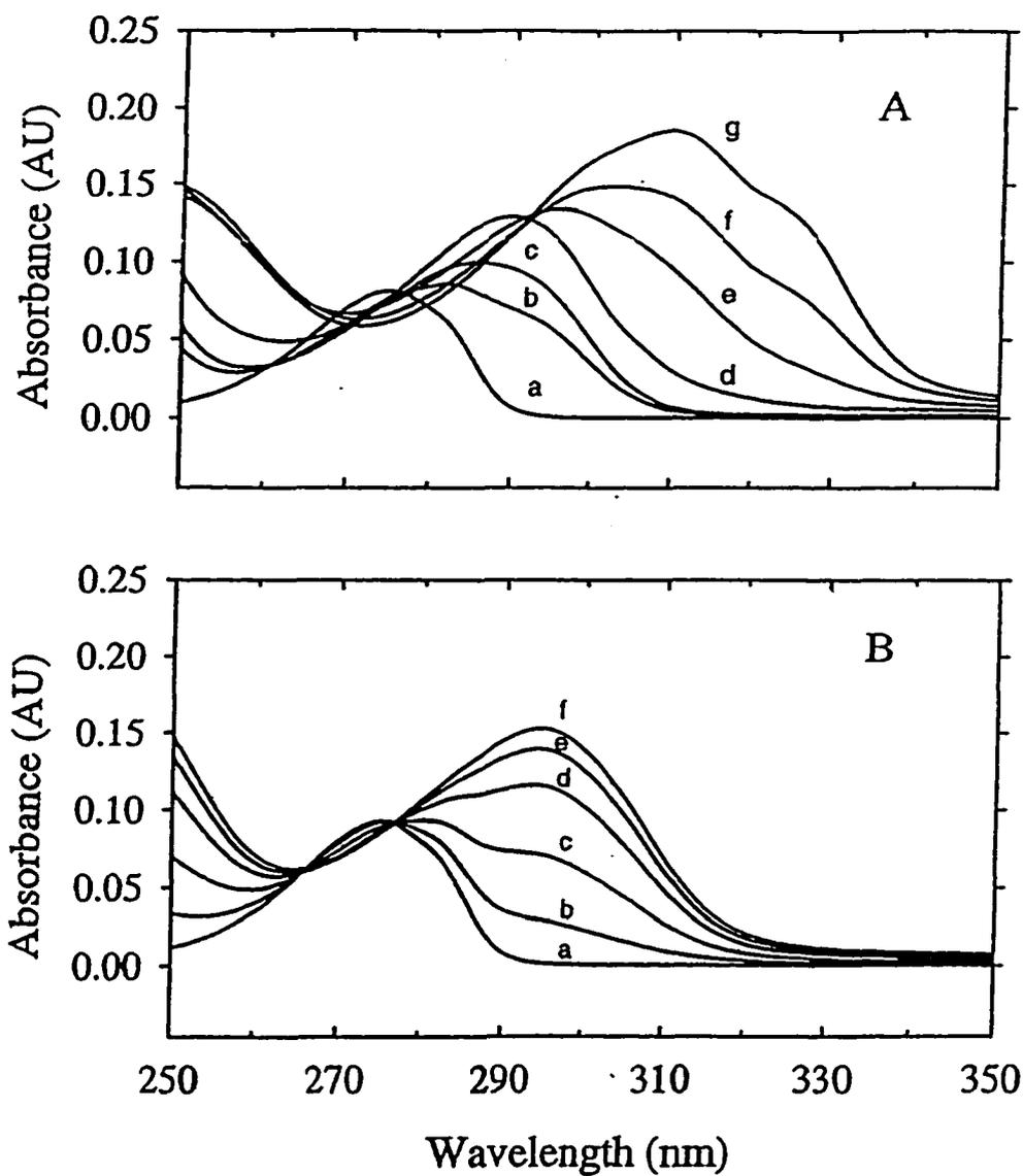
**Figure 1.** Absorption spectra for 0.1 M  $\text{LiClO}_4$  aqueous buffer solutions containing (A)  $4.0 \times 10^{-5}$  M CAT, (B)  $4.0 \times 10^{-5}$  M CAT and  $4.0 \times 10^{-5}$  M  $\text{CoCl}_2$  at several pH values: A. (a) 2.9, (b) 9.6, (c) 10.1, (d) 12.6, (e) 13.1, (f) 13.4, and (g) 13.7; B. (a) 3.0, (b) 8.4, (c) 8.8, (d) 9.1, (e) 9.4, and (f) 9.6.
