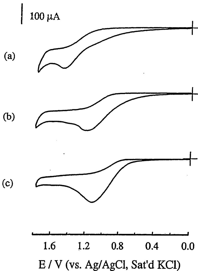
**Figure 1.** Cyclic voltammograms obtained at freshly polished GCEs in ethanolic 0.1 M  $\text{LiClO}_4$  solutions containing 2 mM of (a) butylamine, (b) *N*-ethylbutylamine, and (c) triethylamine. The scan rate was 10 mV/s in each case.
