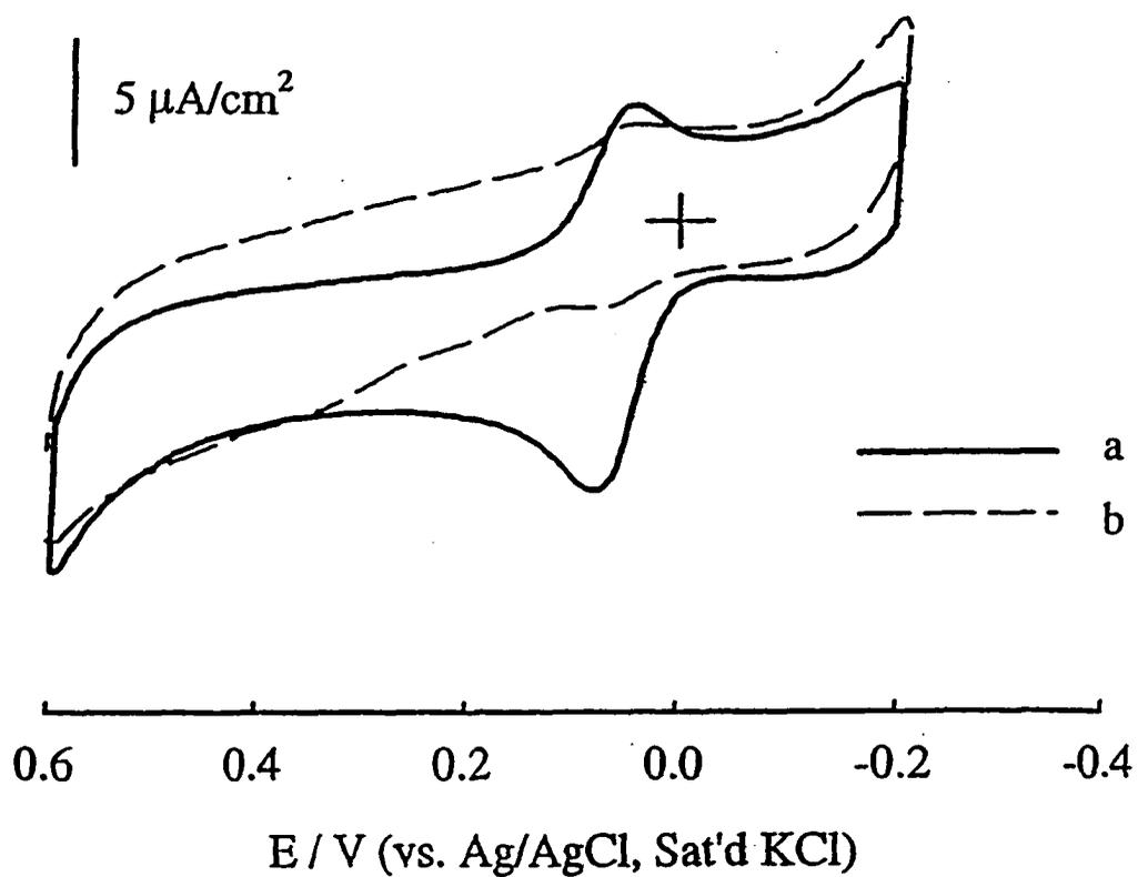
**Figure 2.** Cyclic voltammograms obtained at freshly polished GCEs in aqueous 0.5 M  $\text{LiClO}_4$  buffer solution (pH  $\sim$  9.1) for (a)  $4.0 \times 10^{-5}$  M CAT, and (b) solution a plus  $4.0 \times 10^{-5}$  M  $\text{CoCl}_2$ . The scan rate was 20 mV/s.
