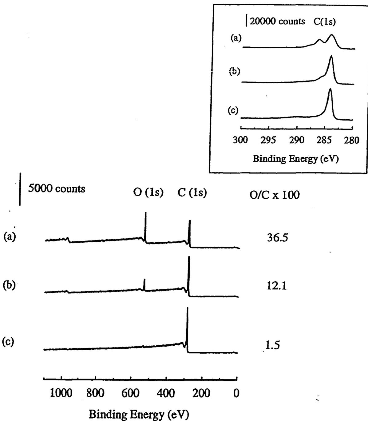
**Figure 3.** X-ray photoelectron survey spectra for (a) electrochemical pretreated GCE, (b) freshly polished GCE, and (c) vacuum heat treated GCE. The insert in the figure shows corresponding high resolution C(1s) spectra.
