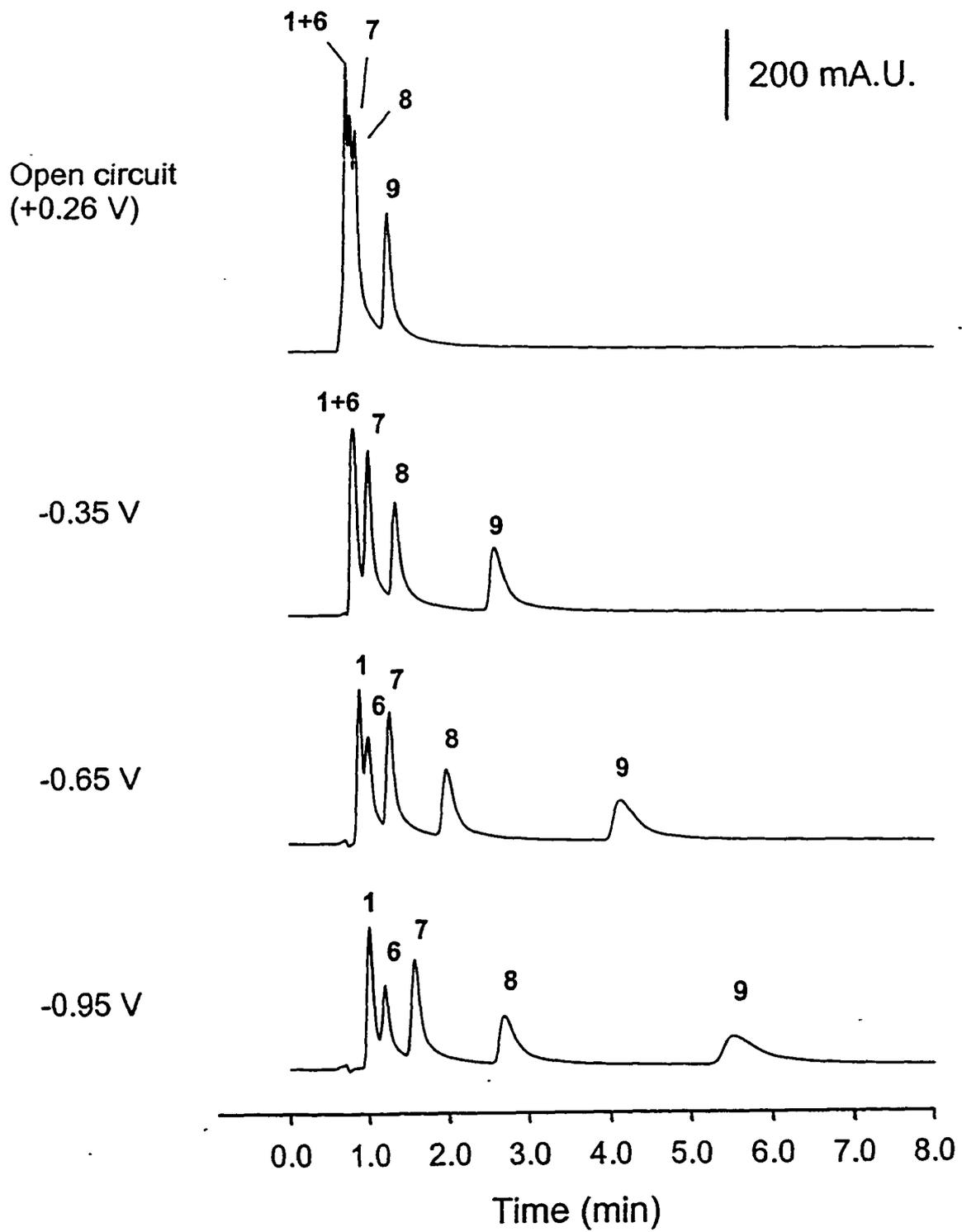
are strongly overlapped at the open circuit potential, whereas a well-resolved separation of all compounds is obtained at  $-0.95$  V with the exception of 1 and 6 which are not fully resolved.
