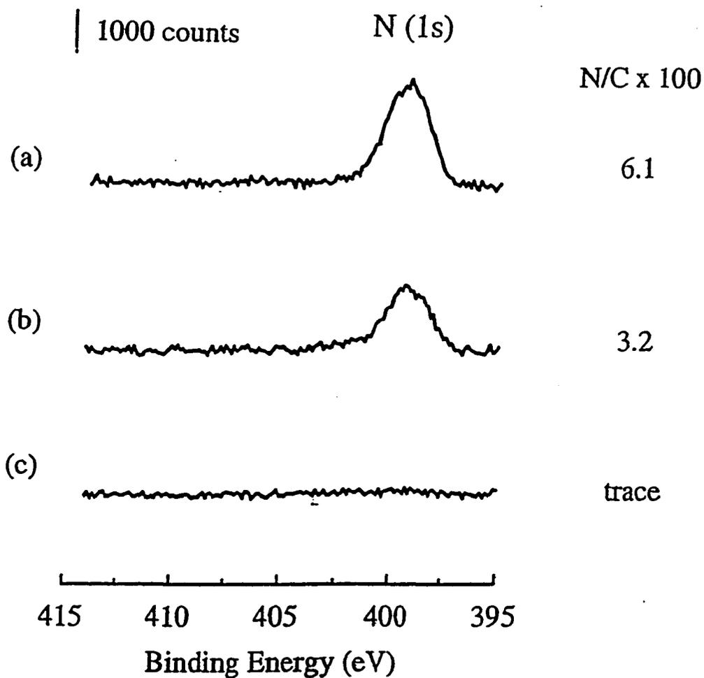
**Figure 7.** X-ray photoelectron spectra in the N(1s) region for freshly polished GCEs immersed in ethanolic 0.1 M LiClO<sub>4</sub> solutions (ethanol:water, 100:1 (v/v) containing (a) 2 mM phenethylamine (PA) only, (b) solution a plus 1.0 mM HClO<sub>4</sub>, and (c) solution a plus 3.0 mM HClO<sub>4</sub>. The applied voltage was cycled once between 0.00 V and +1.80 V at 10 mV/s in each case. The exposure time of GCEs to DA solutions is ~15 min.
