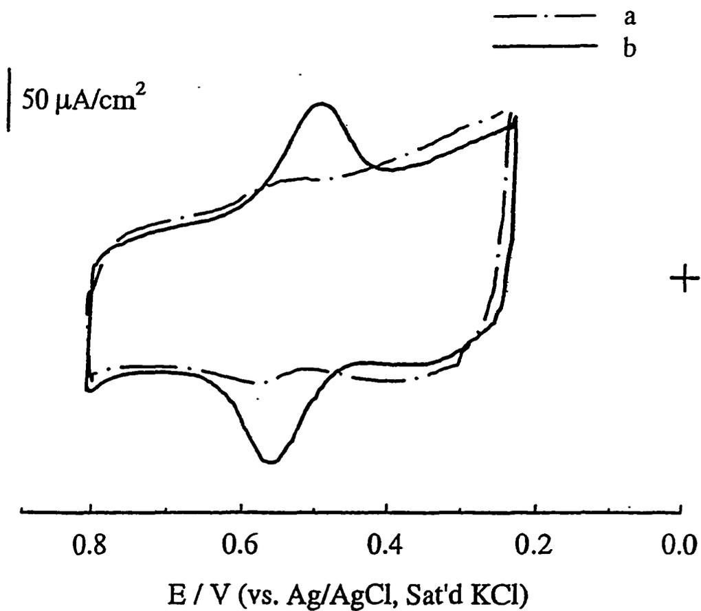
Figure 11. Cyclic voltammograms obtained in aqueous 0.1 M  $\text{HClO}_4$  at DA-modified GCEs from (a) Figure 10a and (b) Figure 10b. The scan rate was 100 mV/s.
