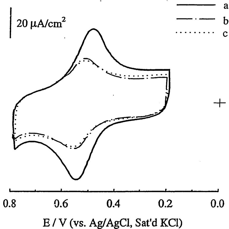
**Figure 3.** Cyclic voltammograms obtained in aqueous 0.1 M HClO<sub>4</sub> solution for dopamine adsorbed on GCE in different pH solution: (a) 9.5, (b) 7.0, and (c) 2.0. The scan rate was 100 mV/s.
